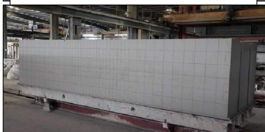
Wire Cutting of processed semi-solid Mixture
